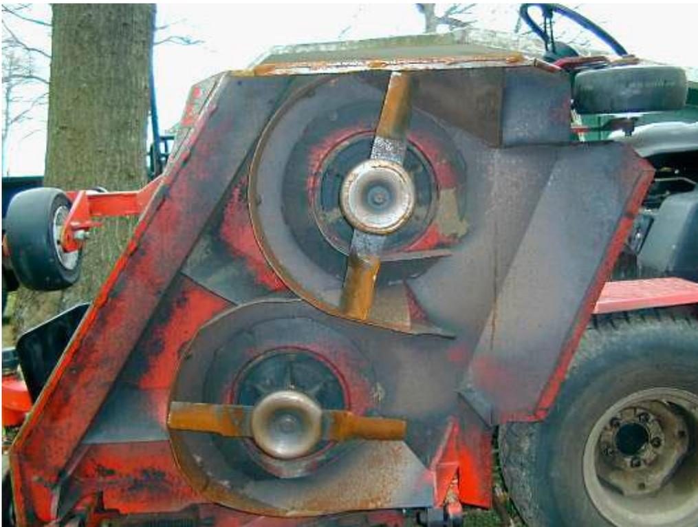
Rotary mowers are best used for height of cuts above 1". Blades should be sharpened after every 10 hours of use. *Source: Frank Rossi.*
