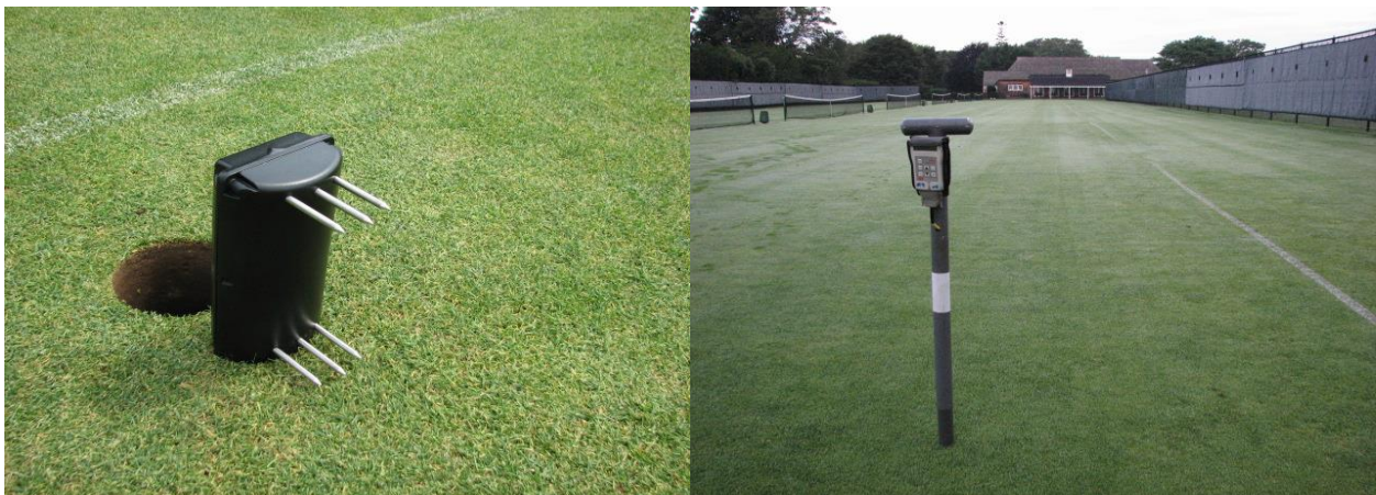
Root zone moisture, temperature, and salinity meter (left) and portable moisture meter (right). Source: John J. Genovesi, Maidstone Club
