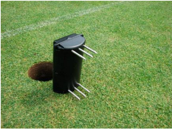
Root zone moisture,temperature, and salinity meter (left) and portable moisture meter (right). Source: John J. Genovesi, Maidstone Club
