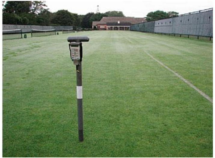
Root zone moisture,temperature, and salinity meter (left) and portable moisture meter (right). Source: John J. Genovesi, Maidstone Club
