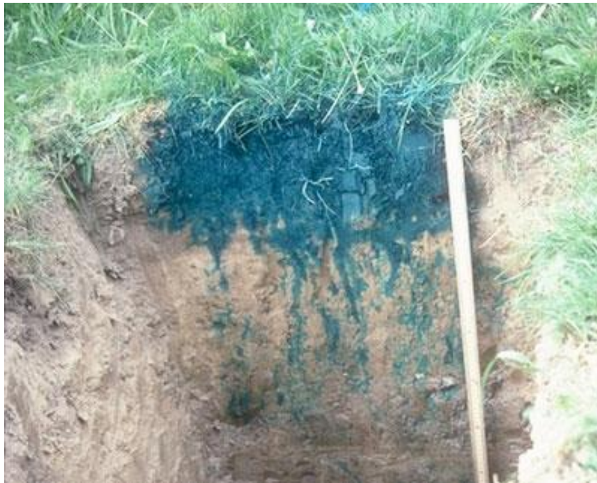
Preferential flow in soils. Source: Cornell, Soil & Water Lab.
